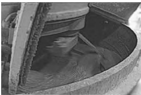
FIGURE 24.9 Various processing methods of ECC: (a) self-consolidating casting, (b) extrusion, (c) spraying, (d) precast mixing (photograph courtesy of S. Staniski) and precasted element.
