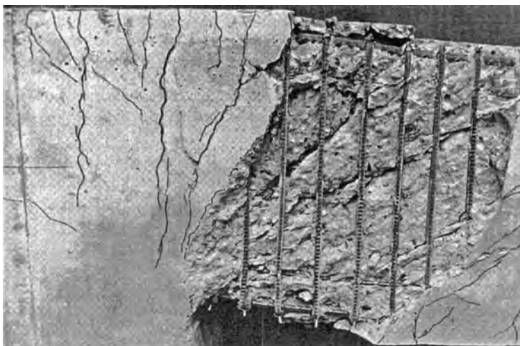
FIGURE 34.8 Compression fan at interior support of the beam, monotonic loading. (From McGregor, J., Reinforced Concrete: Mechanics and Design , 3rd ed., Pearson Education, Upper Saddle River, NJ, 1997. With permission.)
