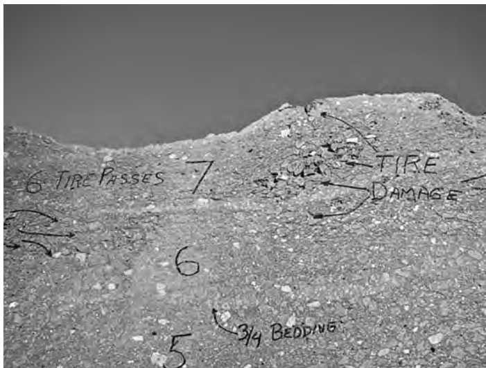
FIGURE 20.17 Interior damage caused by truck traffic on wet-mix RCC.
