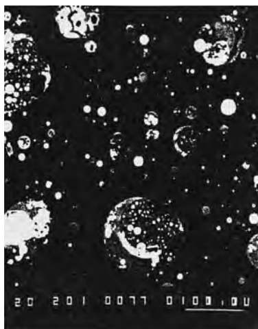
FIGURE 2.2 SEM micrograph of a subbituminous ash: backscattered electron image of a polished section of the dispersed sample. (From Malhotra, V.M. and Ramezaniapour, A.A., Fly Ash in Concrete , MSL 94-45(IR), Canada Center for Mineral and Energy Technology (CANMET), Ottawa, 1994.)
