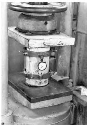
PHOTO 6.4 Cylinder compressive-strength testing set-up.
