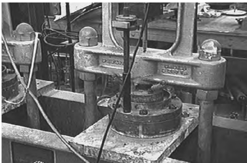
FIGURE 14.21 Laboratory consolidometer apparatus. (Figure courtesy of the University of South Florida, Tampa.)
