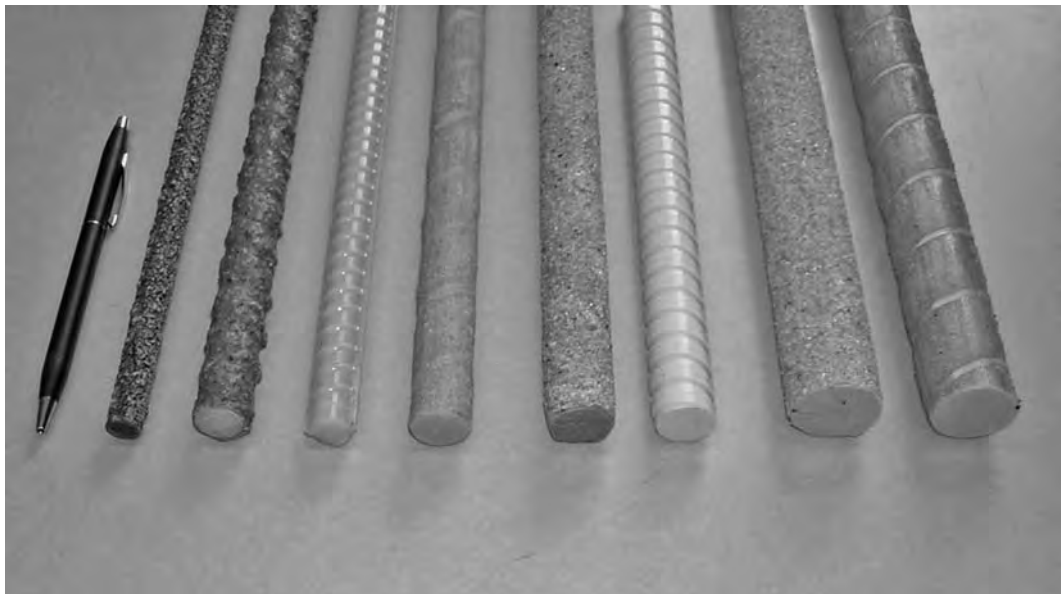
Typical FRP reinforcing bars for concrete members.
