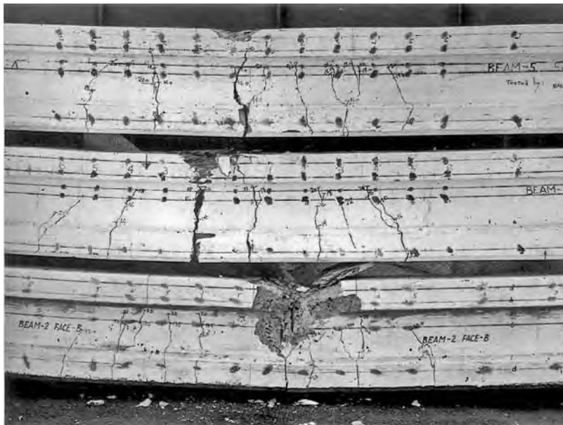
Flexural cracking at ultimate load of post-tensioned prestressed beams. (Photograph courtesy of Edward G. Nawy.)
