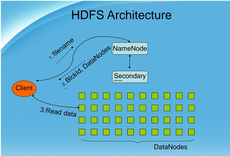
NameNode : Maps a file to a file-id and list of MapNodes DataNode : Maps a block-id to a physical location on disk
