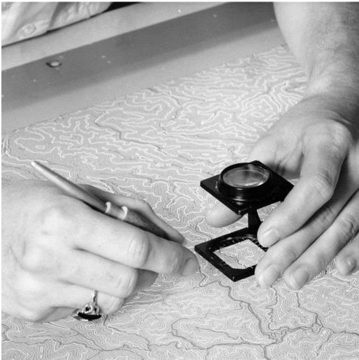
Before the use of computer cartography, mapmaking was a manual process. Scribing of the intermediate contours for a USGS topographic map using a freehand scriber in 1957. Photo: <u>U.S.</u> <u>Geological Survey</u>. Public domain.
