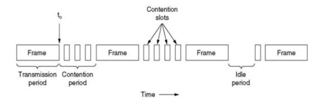
CSMA/CD can be in one of three states: contention, transmission, or idle.
