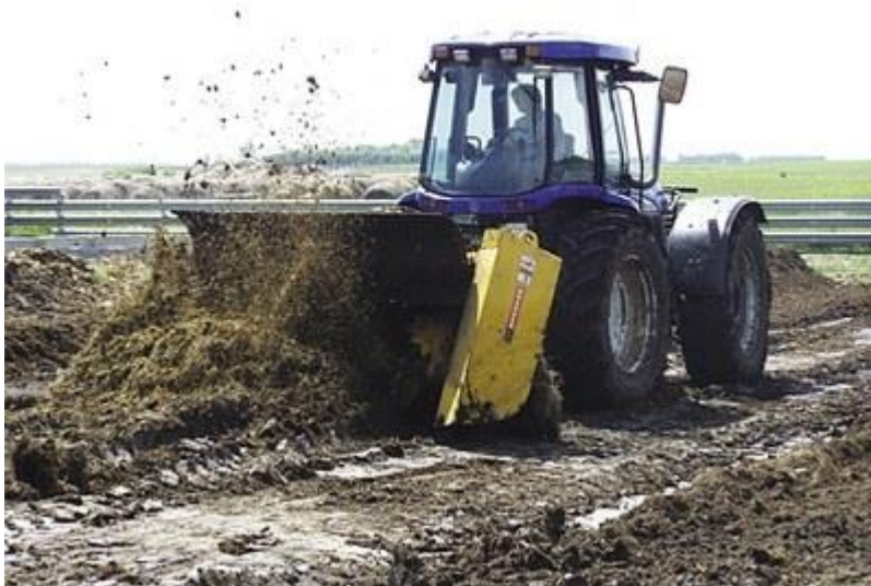
Figure 7. Front-mount composter. This compost turner cleans pens, windrows and turns the pile in the same pass.
