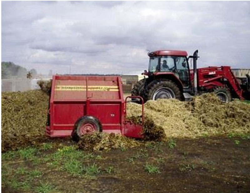
Figure 8. A pull-type compost turner that is turning windrowed bedded feedlot manure for the first time. (photo NDSU Carrington Research Extension Center)
